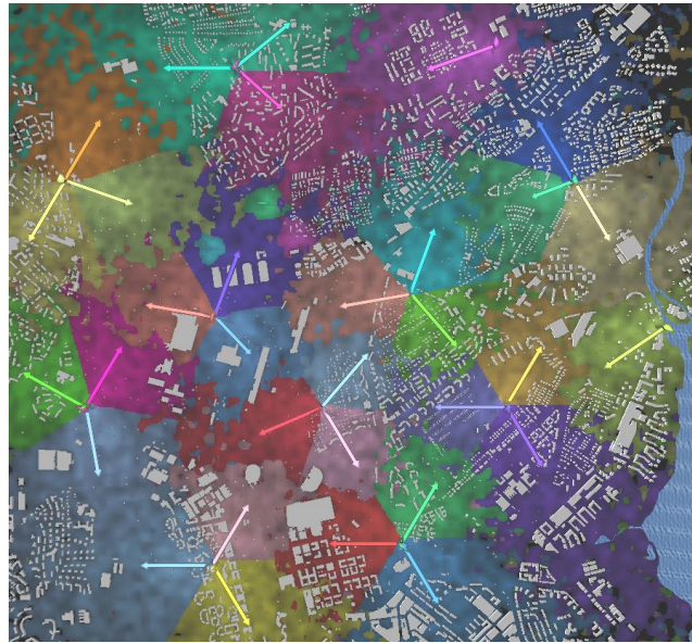
Figure 2.1: Exemplary LTE mobile network with mostly 3-sector BSs taken from the simulation system presented in Chapter 7.2.
