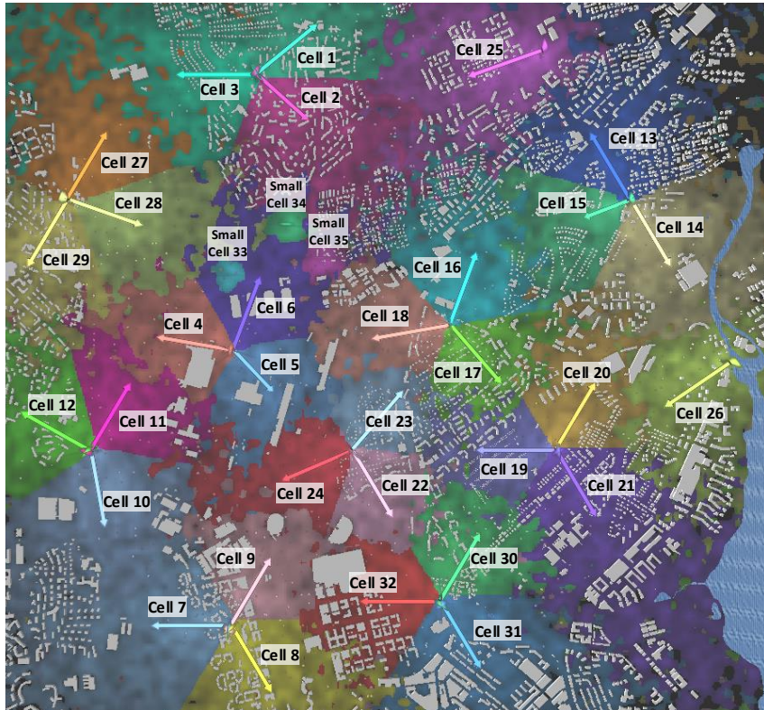
Figure 7.3: Screenshot from the network simulator showing the considered LTE network. The colored patches indicate the coverage areas and the arrows show the main sending direction of the network cells' antennas.
