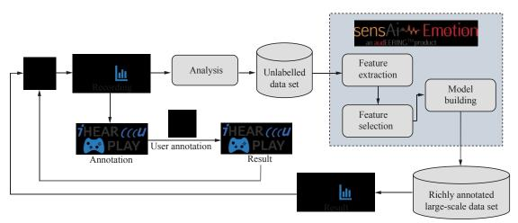
Fig. 2 Schematic overview of the integration of the different VoiLA components into the iHEARu-PLAY crowdsourcing platform for annotation, training and classification of speech
