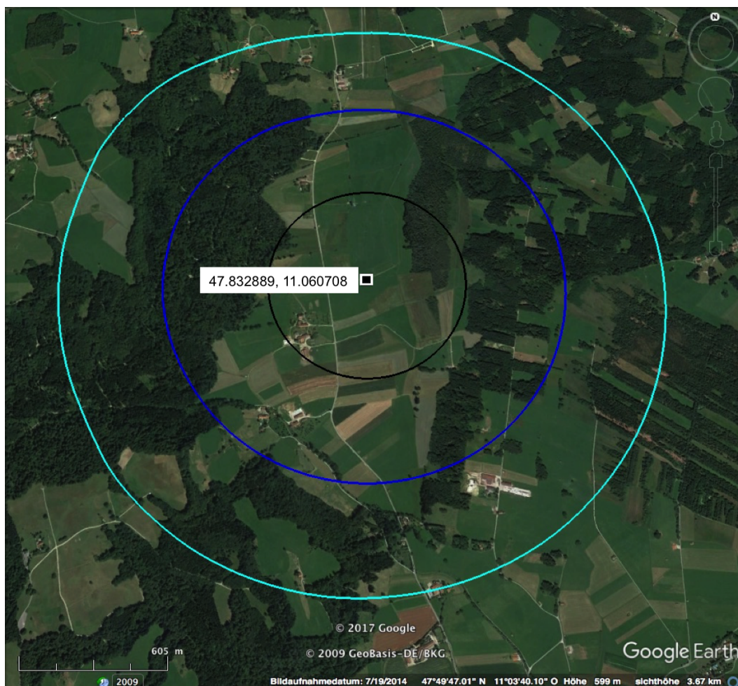
Fig. 7.9: Major contribution areas to cumulative footprints to flux estimation. The black circle has a radius of 500 m around the measured profile, the blue 1000 m and the light blue 1500 m.
