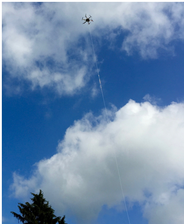
Fig. 3.5: Hexacopter F550 with 70 m tube at about 20 m above ground (Picture taken by Klaus Schäfer).
