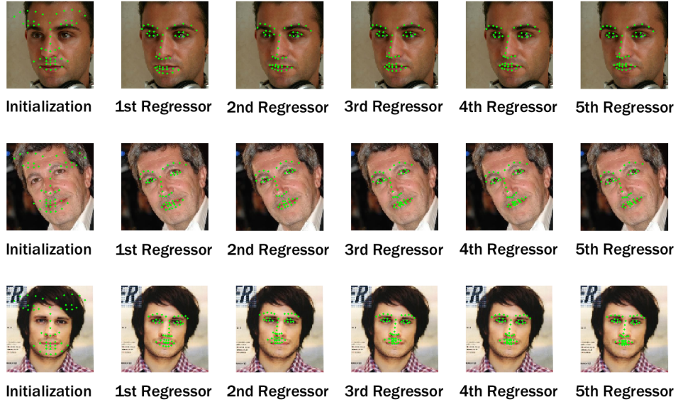
Figure 3.3: Illustration of the iterative process by which the landmarks' set of points is adapted at each layer of the regressor until reaching a distribution close to their real position. Despite this figure being own developed, original images were extracted from ICCV2013 Challenge Database [1].
