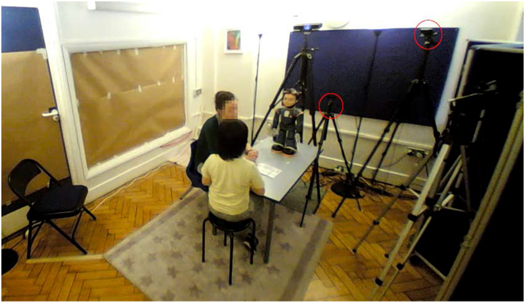
Fig. 2. The experimental setup. The school's staff member who accompanied the child would sit behind the child in the corner of the room. The red circles outline the camera's that were used for annotating our engagement measures, which also included the camera from which this image was taken.
