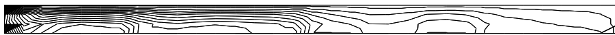
Figure 4.10: Isolines of Stokes velocity modulo of the aggregated problem in the case of sand, cross section y = 10 .
