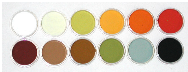
Figure 4.2: Picture showing the colors of different compounds. Top line (from left to right): TiO_2 , TiO_xN_y , CaTaO_2N , Sr_2TaO_3N , SrTaO_2N , NdTaO_2N . Bottom line: BaTaO_2N , EuTaON_2 , LaTiO_2N , Yb_2Ta_2O_5N_2 , SrTiO_3:N and BaNbO_2N .
