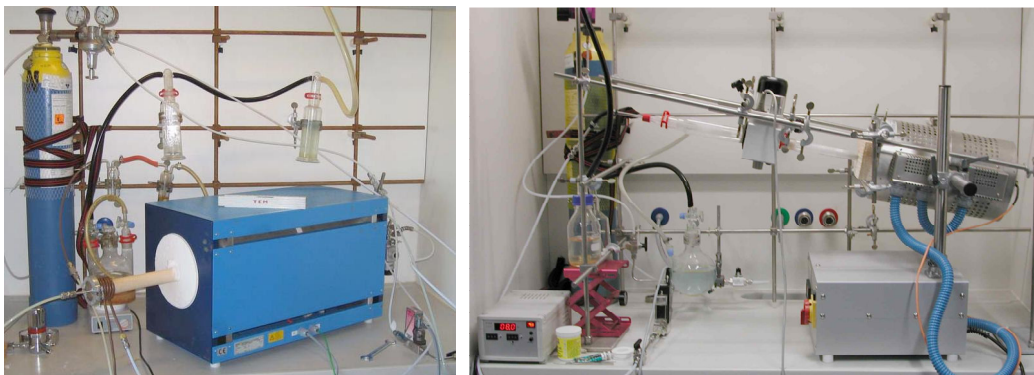
Figure 3.1: Pictures of static (left) and rotating (right) tube furnaces used for ammonolysis.
