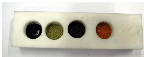
Figure 2.5. Photograph of the self built Al 2 O 3 sample holder used for the screening experiments.
