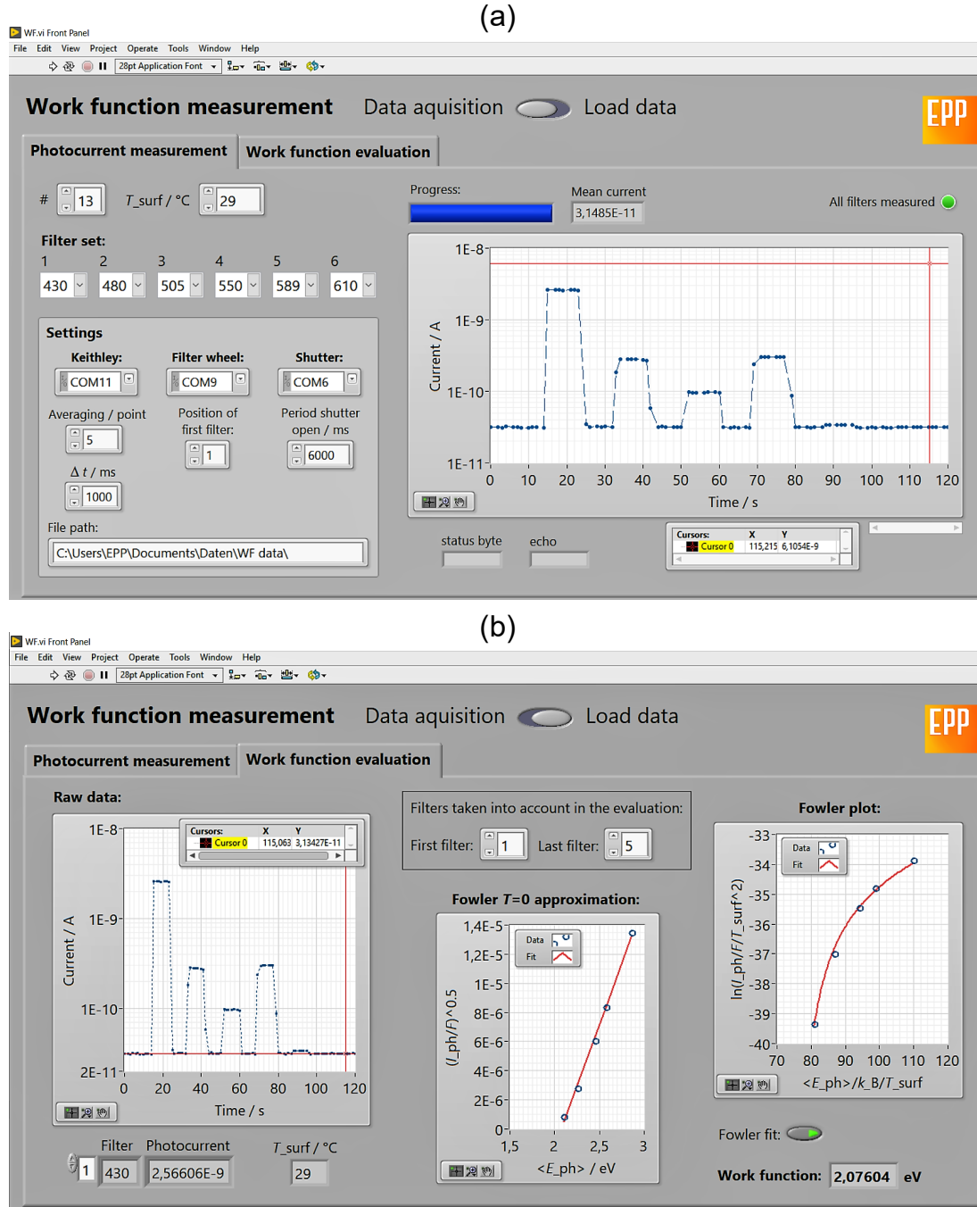
Figure 6.3: Graphical user interface of the work function measurement program developed with LabVIEW. The tabs for the photocurrent measurement and the work function evaluation via the Fowler method are shown in (a) and (b), respectively.
