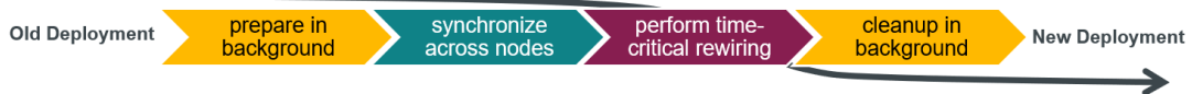
FIGURE 4.2: Overview of the basic phases of a reconfiguration. The reconfiguration is prepared in background (e.g. downloading and starting new containers). Then the involved nodes notify each other to synchronously perform the time-critical modifications (e.g. activating tasks, transferring state, ...). Finally, the reconfiguration is finalized in background (e.g. stopping old containers).
