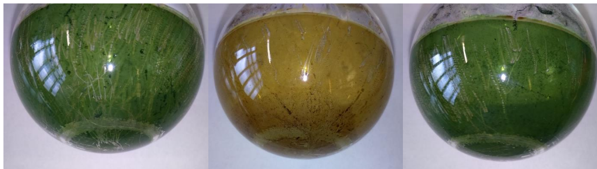
Figure S53. Photographs of CFA-19 (left) in a MeOH atmosphere (middle) and after a few seconds of vacuum drying (right) showing the intense and rapid color change from green to golden to green due to the change in the coordination environment of the peripheral cobalt ions from tetrahedral to octahedral to tetrahedral
