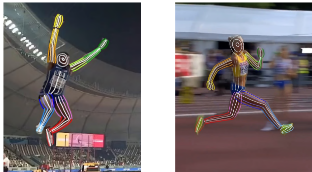
Figure 1. Two detection results of arbitrary keypoints on images of our jump-broadcast dataset using our model, visualized with three equally spaced lines to both sides of each body part including the outer boundary in pure color and the central line in white with a color gradient from the boundary to the central line.
