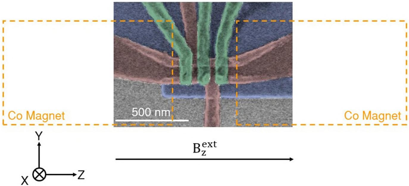
**Extended Data Figure 1 | Micromagnet design.** To-scale drawing of the micromagnet design, superimposed on top of the SEM image of the DQD. The coordinate axes and the direction of the externally applied magnetic field  $B_z^{\text{ext}}$  are indicated at the bottom. In this geometry, the DQD electron experiences a homogeneous  $z$  field  $B_z \approx B_z^{\text{ext}} + B_z^{\text{M}}$ . The total  $x$  field  $B_x$  that
