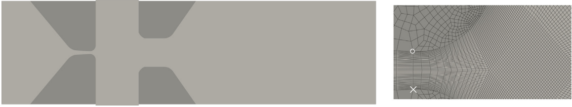
Fig. 19. Human phonation example: computational domain considered (left) and close-up of the mesh on the top VFs' trailing edge (right) with points A (x) and B (o) highlighted.
