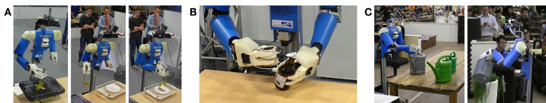
FIGURE 11 | Tool use. (A) Grasping sausages with a pair of tongs. Cosero perceives position and orientation of the sausages in RGB-D images (Stückler and Behnke, 2014a). (B) Bottle opening. (C) Plant watering skill transfer to unknown watering can (Stückler and Behnke, 2014b; cf. to Figure 8E ).
