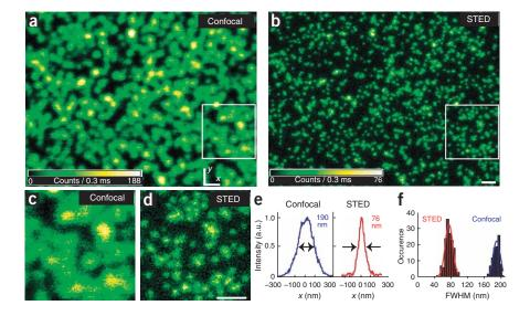
Figure 2 | STED overcomes the diffraction resolution barrier in GFP-based microscopy.
