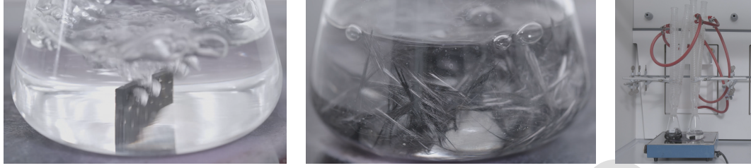
Figure 3: Drop of a specimen in sulfuric acid in Erlenmeier flask and dispersion of the fibers. Courtesy of FIBRE Bremen.
