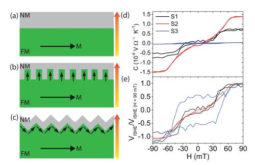
FIG. 4. (a–c) A schematic illustration of the interface morphologies of the NM/FM system for different surface treatments of the FM where orange arrows represent  $\nabla T$ : (a) An atomically flat interface, (b) an interface with a perpendicular anisotropy and (c) a rough interface. (d) Comparison between the magnitude of the C parameter and (e) comparison between the line profile of the SSE signal as a function of H for all samples.
