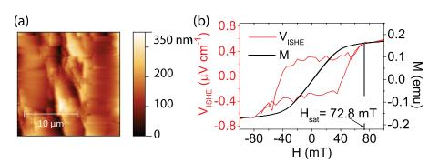
FIG. 3. (a) AFM height image of the YIG surface for sample S3  $(20 \times 20 \,\mu\text{m}^2)$  and (b) a comparison between the H dependence of  $V_{\rm ISHE}$  at  $\Delta T = 7.5 \text{ K}$  in sample S3 and the magnetization M of the YIG crystal.
