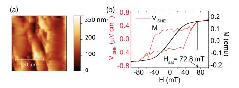
FIG. 3. (a) AFM height image of the YIG surface for sample S3  $(20\times20\,\mu\mathrm{m}^2)$  and (b) a comparison between the H dependence of  $V_{\mathrm{ISHE}}$  at  $\Delta\mathrm{T}=7.5\,\mathrm{K}$  in sample S3 and the magnetization M of the YIG crystal.
