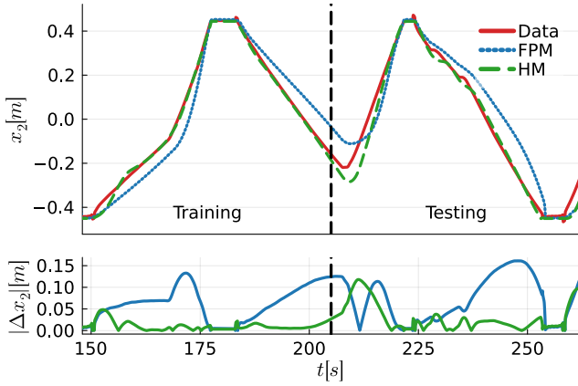
Figure 12. Comparison of bucket cylinder position to data (top) and absolute deviation from data (bottom). The HM is modeled on basis of the FPM with simple friction.
