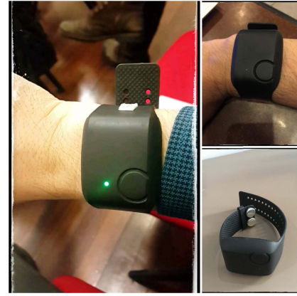
Fig. 5. The data collection device is shown. The electrodes in the bottom right image are for EDA sensors. PPG and ST sensors are presented in the bottom middle image.
