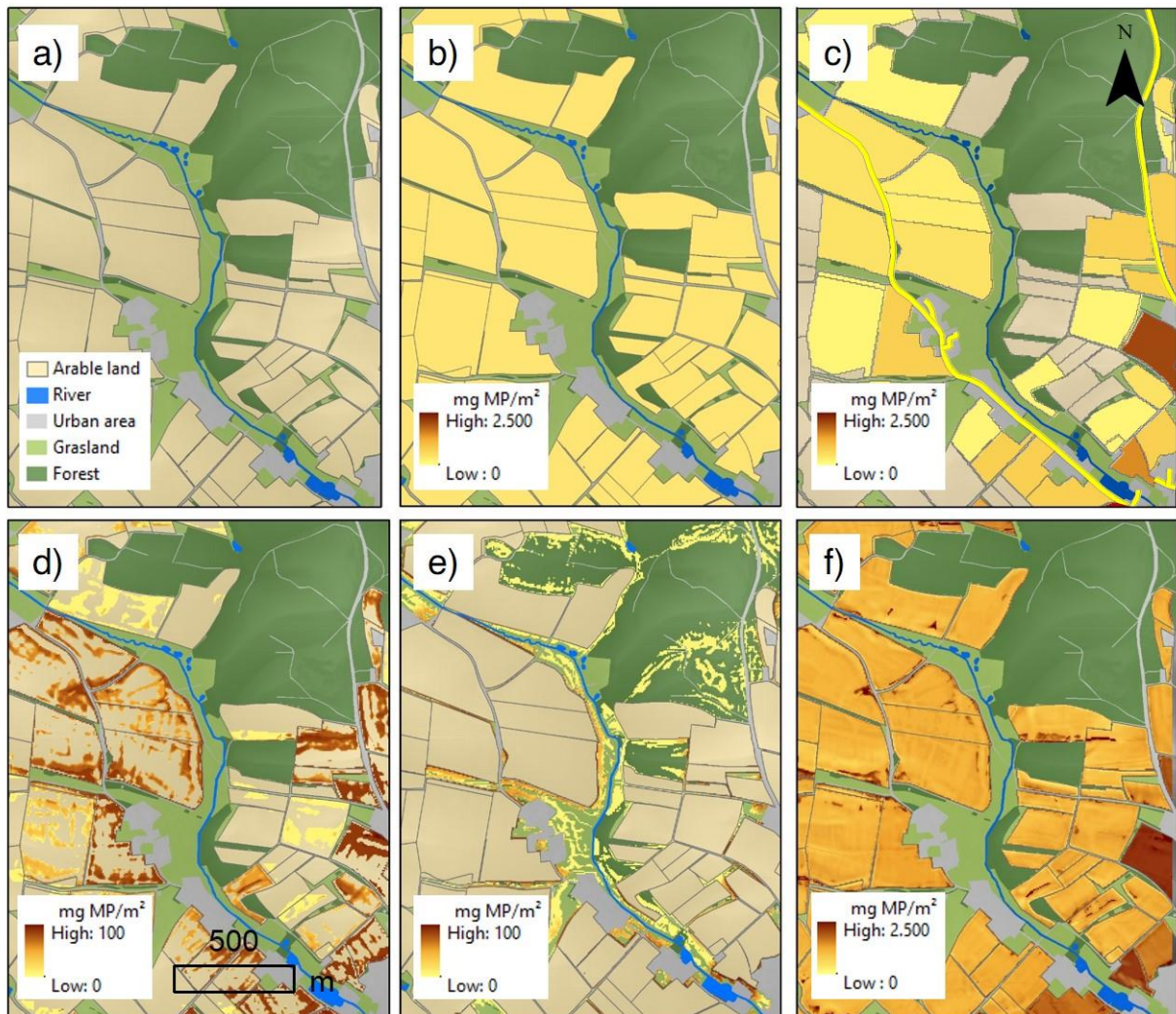
Figure 15: Example of catchment segment (for location, see Figure 10) illustrating microplastic (MP) input on arable land and results of erosion modeling between 1950 and 2020. The maps show the situation in 2020. a) Field-based land use. b) Total MP input from sewage sludge, compost, and atmospheric input (without TW) as a mean value over all arable land. c) MP input from TW, spatially distributed to individual arable fields along the roads. d) MP concentration below the plough layer. e) MP transported to other land uses via soil erosion. f) MP distribution after water and tillage erosion on arable land.
