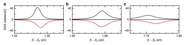
Figure 5 | DOS for the three LUMOs of a representative Alq<sub>3</sub> molecule in the second layer. Panel (a) corresponds to the LUMO with a large contribution from N'<sub>1</sub>, (b) with a large contribution from N'<sub>2</sub> and (c) with a large contribution from N'<sub>3</sub>.
