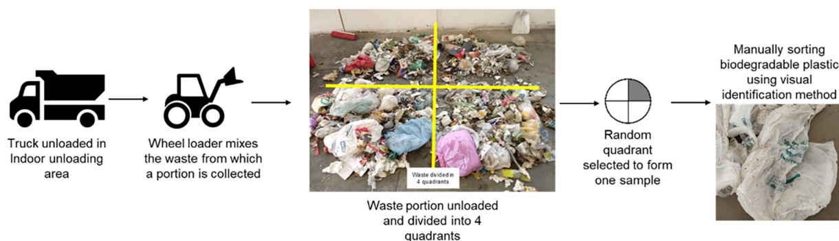
Figure 3. Sampling of residual waste in a splitting plant in Austria.
