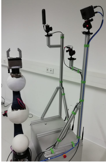
Figure 4.1. Photo of the camera rack and the mounted cameras.
