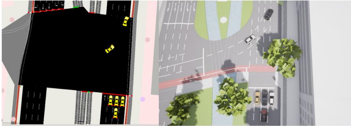
Figure 2 Interfacing an ongoing SUMO simulation (left) into a 3D VR environment in Unity (right).
