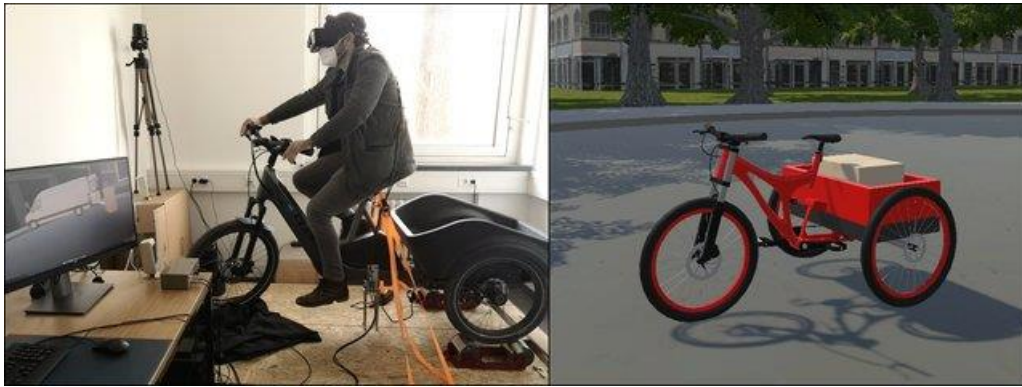
Figure 4 Depiction of a test subject operating the electric cargo bicycle simulator with typical sensor setup and usage of a Varjo XR-3 (left) and of the virtual electric cargo bicycle in VR environment in Unity (right).
