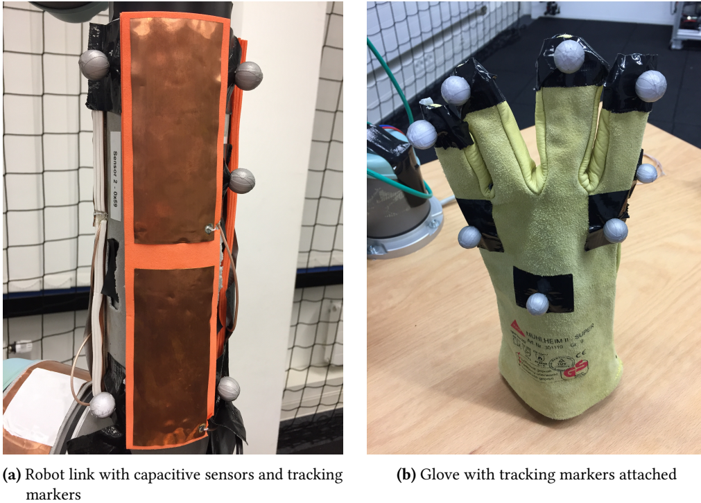
Figure 5.10. Capacitive sensors and marker setup for the robot arm and glove to be worn during data recording in order to determine the ground truth distance values for later training of the neural net.
