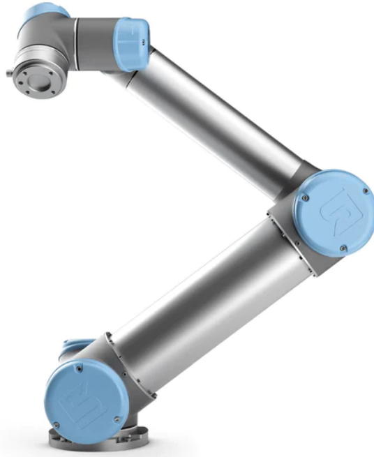
Figure 5.11. The UR5 robot from Universal Robots. A collaborative robot with six axes, capable of manipulating a payload of up to 5kg in the vicinity of humans. Due to its simple geometric construction it is a popular choice for researches seeking to mount additional hardware to a robot quickly and easily. (Image source: [119])
