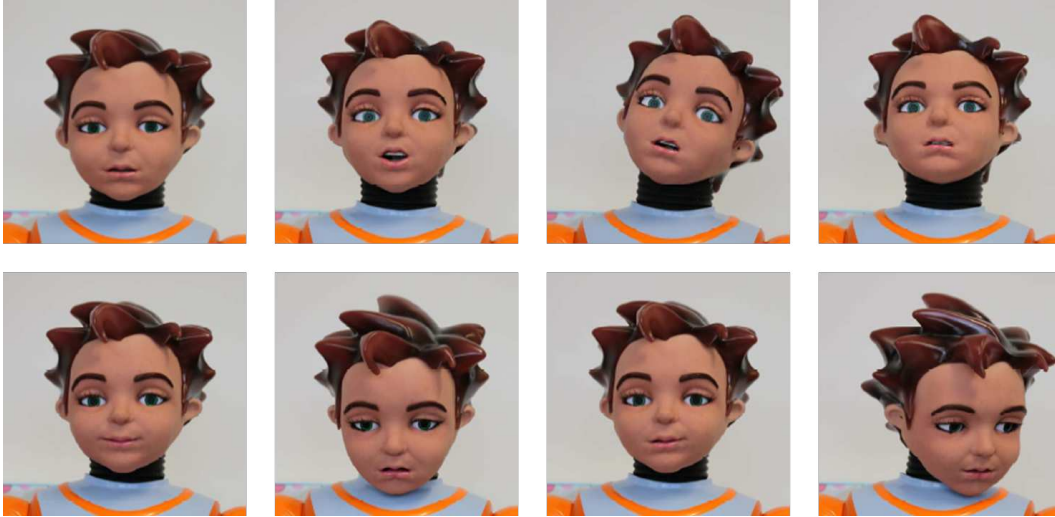
Figure 8.4: Facial expressions of the RoboKind R-50 Zenon. From top left to bottom right: Neutral, surprise, fear, anger, happiness, sadness, contempt, shame.
