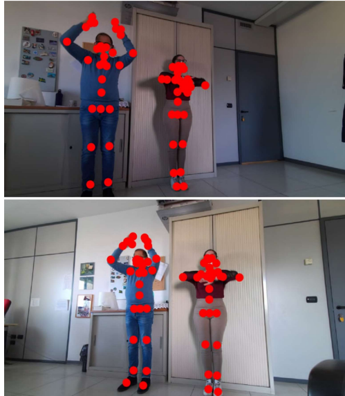
Fig. 3. Two RGB images captured from two synchronized Azure Kinect cameras looking at the same workspace. Here, two users are detected and tracked to obtain the corresponding skeletons.
