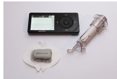
(b) Continuous glucose sensor, transmitter, receiver, and injection aid to measure subcutaneous glucose concentration.
