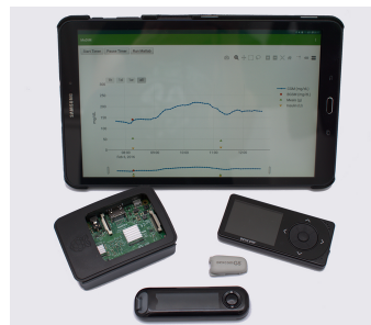
Figure 7.3: MoDiM hardware consists of a tablet device (back), Dexcom G5 Mobile CGM sensor and receiver (front right), Contour Next One blood glucose sensor (front center), and Raspberry Pi (front left).
