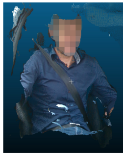
(b) Illustration of recorded data as point cloud in 3d space. Pixels without spacial information are not visualized.
