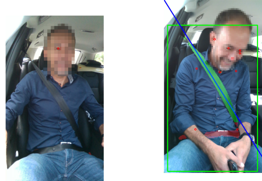
(b) Qualitative example of the key measurement 'position of the head in relation to the head rest'. The image is sampled by filtering the corresponding histogram 'Depth position'.
