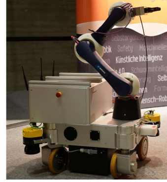
Fig. 4: The robot platform, using a Neobotix MPO-700 platform and Schunk LWA arm. The arm is shown here with a custom sensor casing unrelated to the described research.
