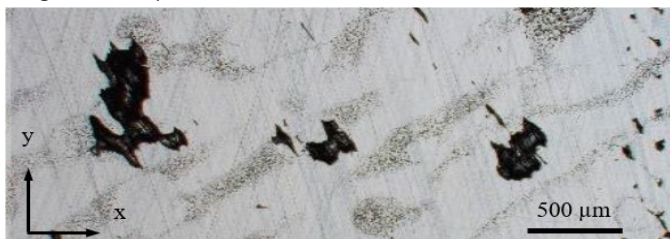
Fig. 5. Horizontal micrograph of artificially inserted defects
