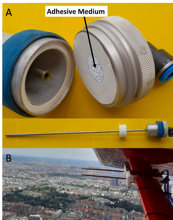
Fig. 2. A. Details of the isokinetic impactor (photo by U. Gosewinkel). B. Two isokinetic impactors employed from the aircraft flying over Copenhagen (photo by M.P. Plaza).
