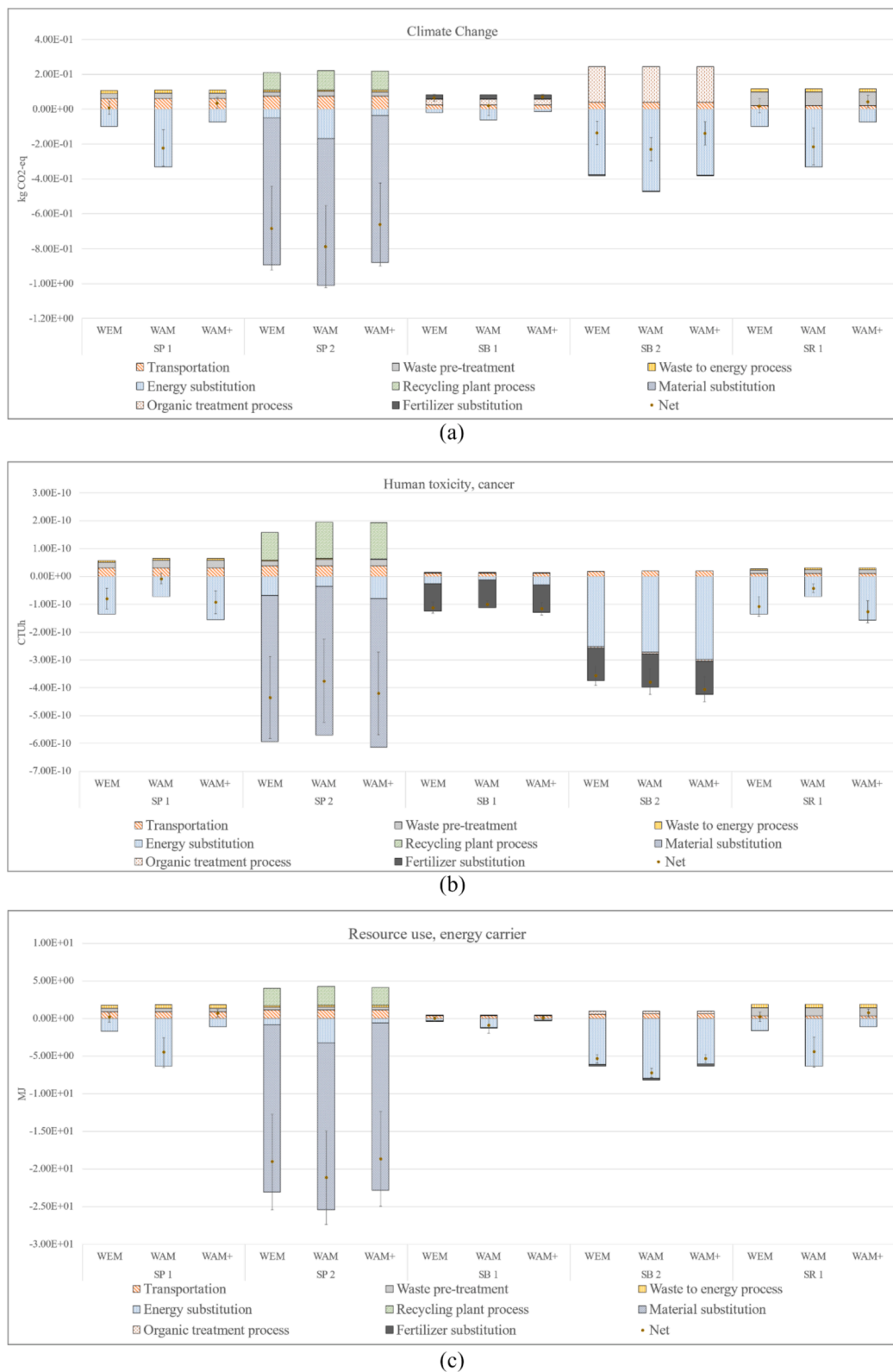
Fig. 5. Results of characterisation for comparison of three energy scenarios (WEM, WAM, WAM +) for the following impact categories (a) Climate change; (b) Human toxicity – cancer; (c) Resource use – energy carrier. Throughout the manuscript, the WEM scenario is considered the default energy scenario. Each coloured stack in an individual bar represents the net value of relevant grouped processes and the net value of the bar is represented by a ‘dot’, where the negative values are termed as savings and the positive values as load. The results of uncertainty propagation were represented by error bars. SP1 – packaging waste pathway plus incineration; SP2 – packaging waste pathway plus mechanical recycling; SB1 – biowaste pathway plus composting; SB2 – biowaste pathway plus anaerobic digestion; SR1 – residual waste pathway plus incineration. Energy scenarios were based on (Baumann & Kalt, 2015), where, WEM – energy scenario with existing measures, baseline energy scenario; WAM – energy scenario with additional measures, reduced electricity imports and heat from natural gas; WAM + energy scenario with additional measures plus, zero electricity imports and heat from biomass.
