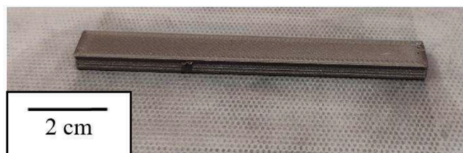
Fig. 1. Specimen manufactured by Markforged's Mark Two 3D printer.
