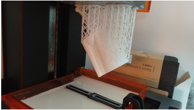
(a) SLA printed object still in the machine.
