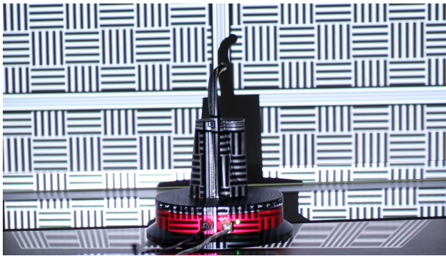
Figure 1: Structured Light scanning. The object is placed on a turntable. The deformations of the light can be seen on the scanned object.
