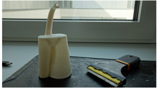
(b) SLA printed object after post-processing.
