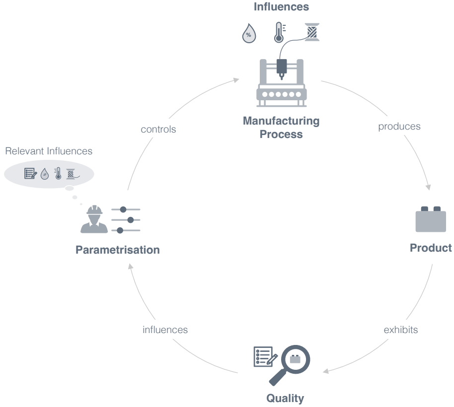
Figure 2.1.: Parametrisation process as encountered in manufacturing.
