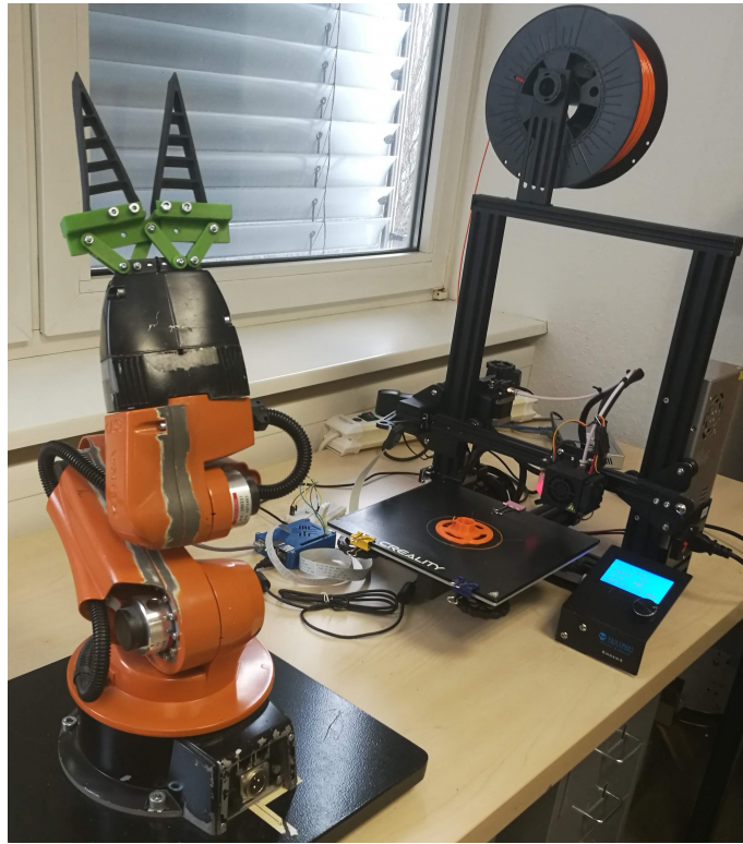
Figure 3.2.: Creality Ender-3 with a KUKA YouBot to automatically extract finished products. Next to the printer the blue Raspberry Pi that controls the printer and measures environmental factors, i.e. temperature and humidity, is visible. Previously published in [Wie+21].
