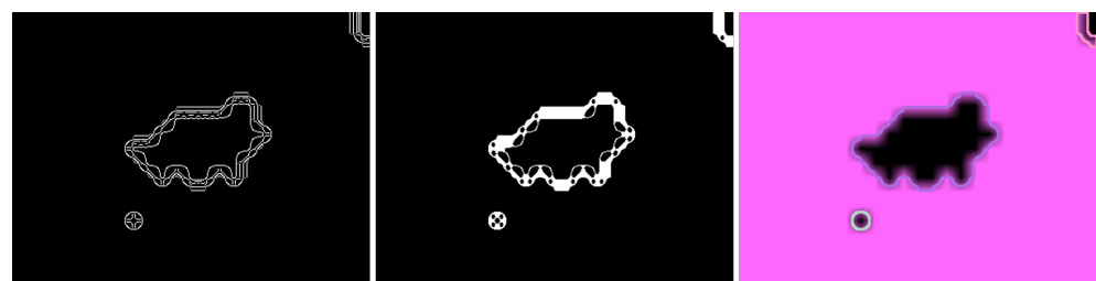
Figure 8. Contour detection pipeline; from left: Canny edge detection, morphologic closing, chain approximation.
