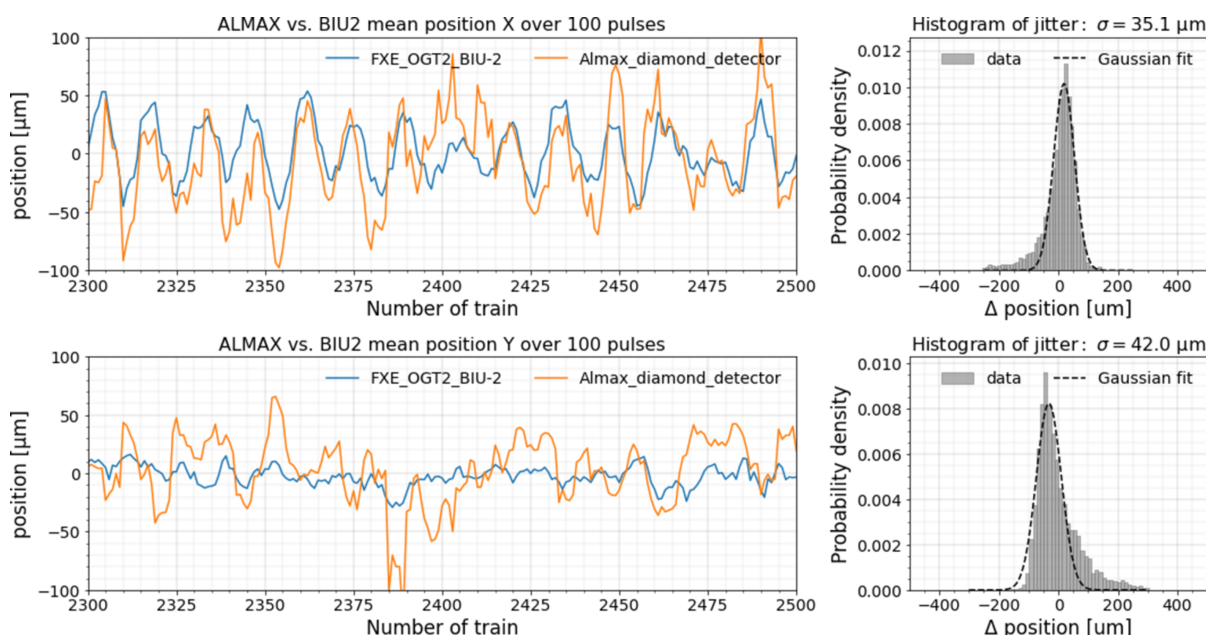
Figure 10 Beam position measured simultaneously in the x - and y -directions by the ALMAX detector and BIU2 for a focused beam. The histograms on the right show the respective deviation in beam positions determined by BIU2 and ALMAX.
