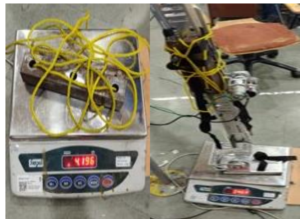
Fig. 16. (a) Weight of metal rod (b) Weight of exoskeleton after attaching metal rod
