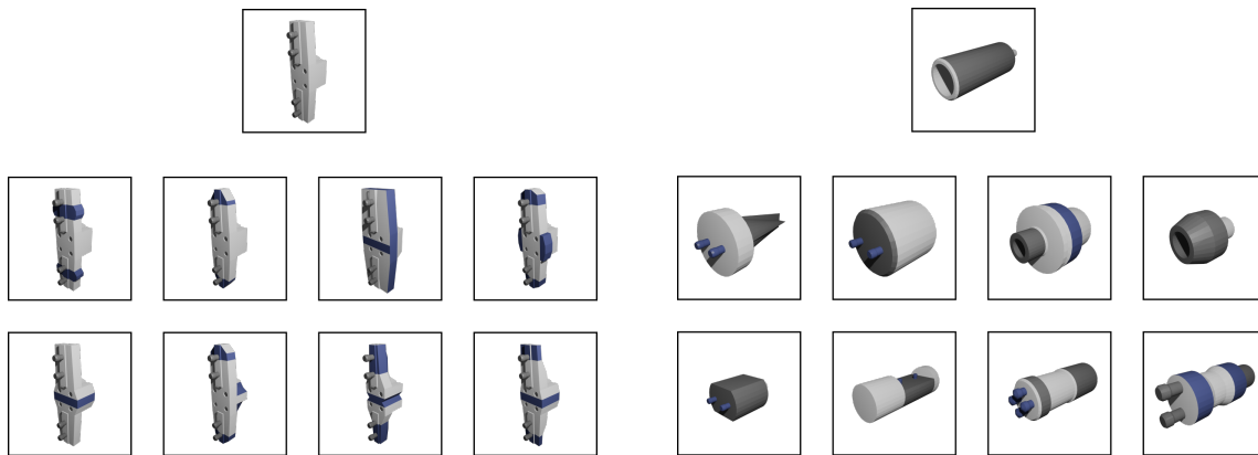
Figure 4.4: Inspection of eight nearest parts to given part (shown centered in first row) in the embedding space – good and bad example for learning similar representations of similar parts shown on the left and right, respectively.
