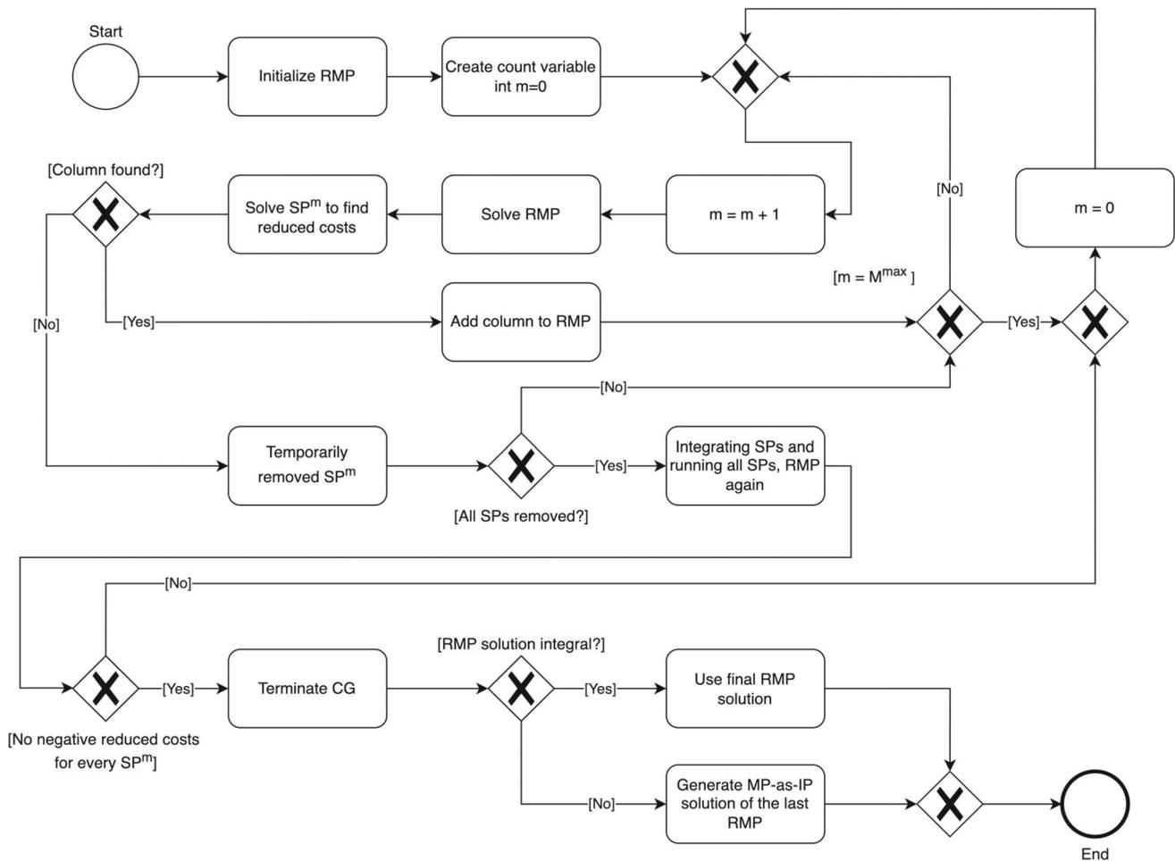
Fig. 3 Column generation (CG) algorithm process flow
