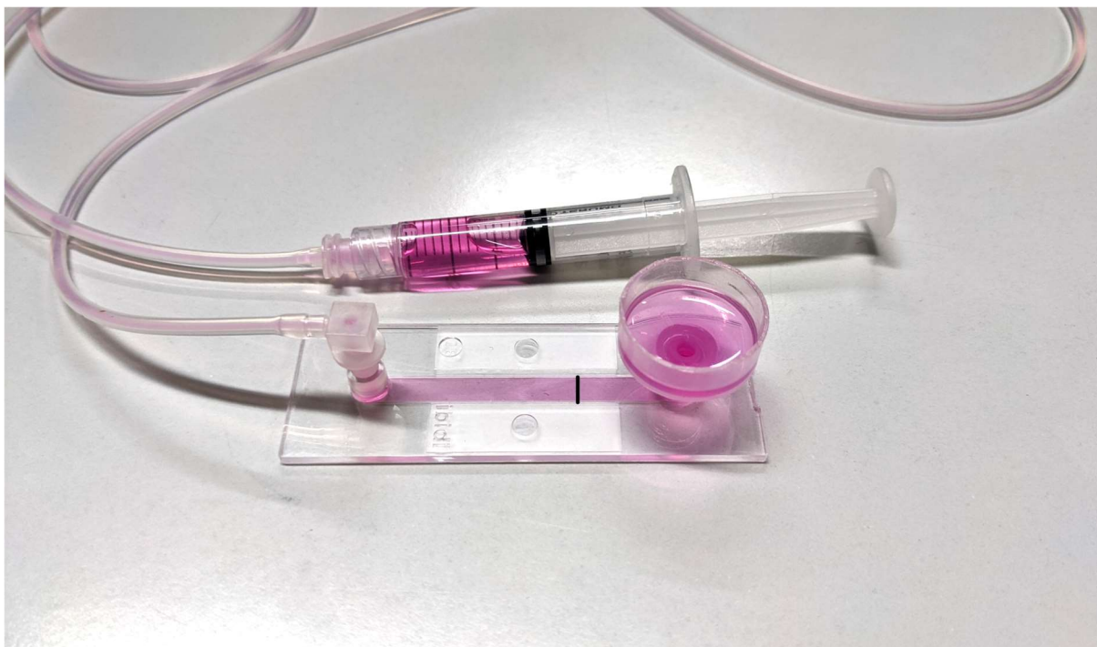
Figure 3.5: Vesicle Reservoir for Adhesion Measurements. A reservoir made from a syringe is connected to one end of a channel slide, filled with a vesicle solution. A tube on the other end of the channel slide is connected to a syringe placed in a syringe pump. The pump operates in reverse mode, sucking the vesicle solution from the reservoir through the channel slide into the syringe.
