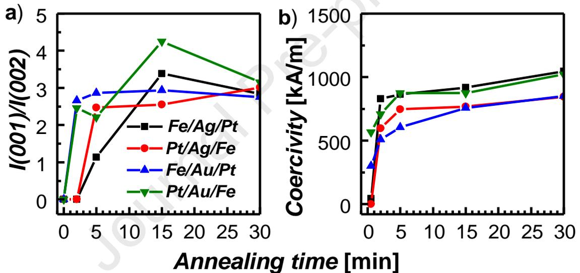
**Fig. 3.** Dependence of (a)  $I(001)/I(002)$  intensity ratio and (b) coercivity of Fe(15 nm)/Ag(Au)/Pt(15 nm) and Pt(15 nm)/Ag(Au)/Fe(15 nm) trilayers after post-annealing at 700 °C on the annealing time.
