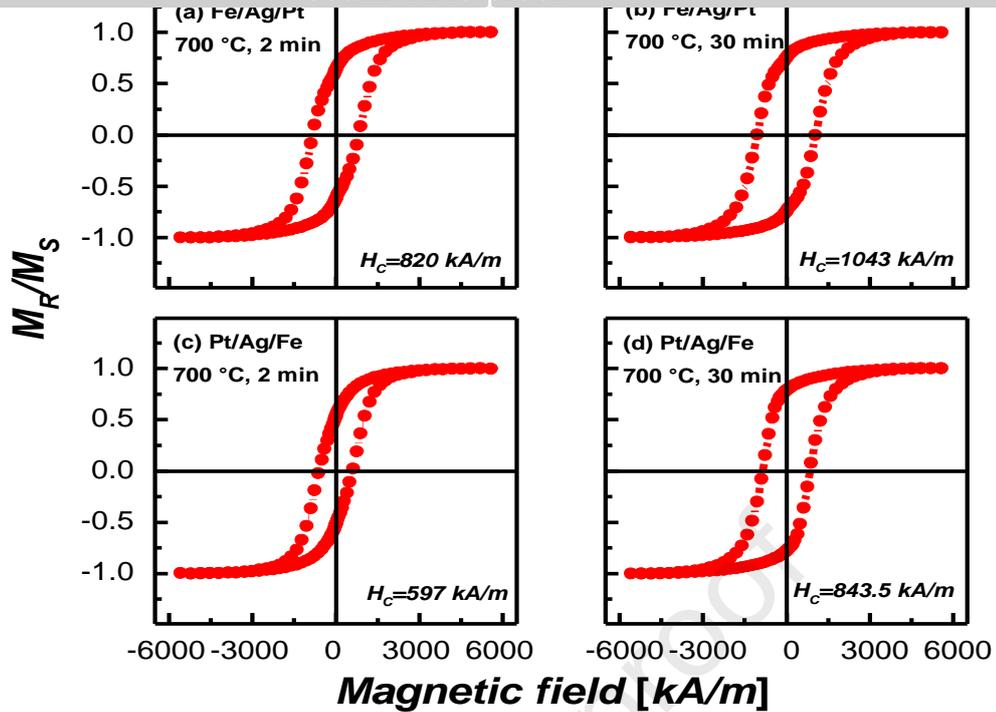
**Fig. 4.** Out-of-plane hysteresis loops of (a, b) Fe(15 nm)/Ag(10 nm)/Pt(15 nm) and (c, d) Pt(15 nm)/Ag(10 nm)/Fe(15 nm) films after post-annealing at 700°C for 2 min and 30 min, respectively.
