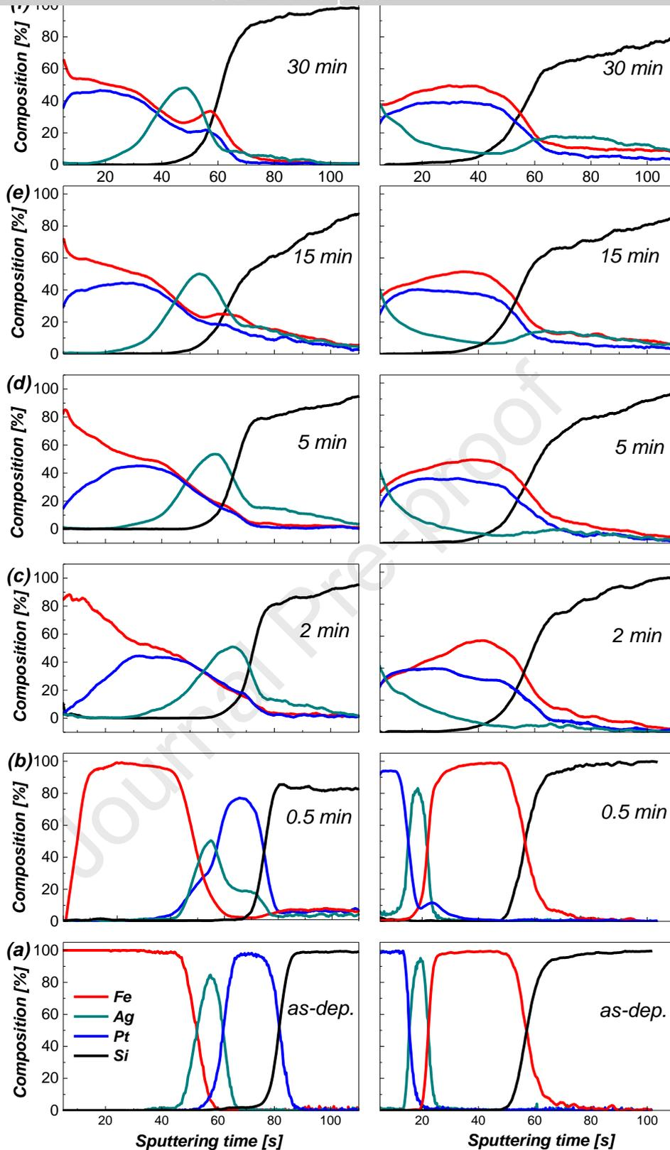
**Fig. 2.** Compositions versus sputtering time profiles of the (a) as-deposited Fe(15 nm)/Ag(10 nm)/Pt(15 nm) and Pt(15 nm)/Ag(10 nm)/Fe(15 nm) trilayers and (b-f) after annealing at 700 °C for different annealing times up to 30 min.
