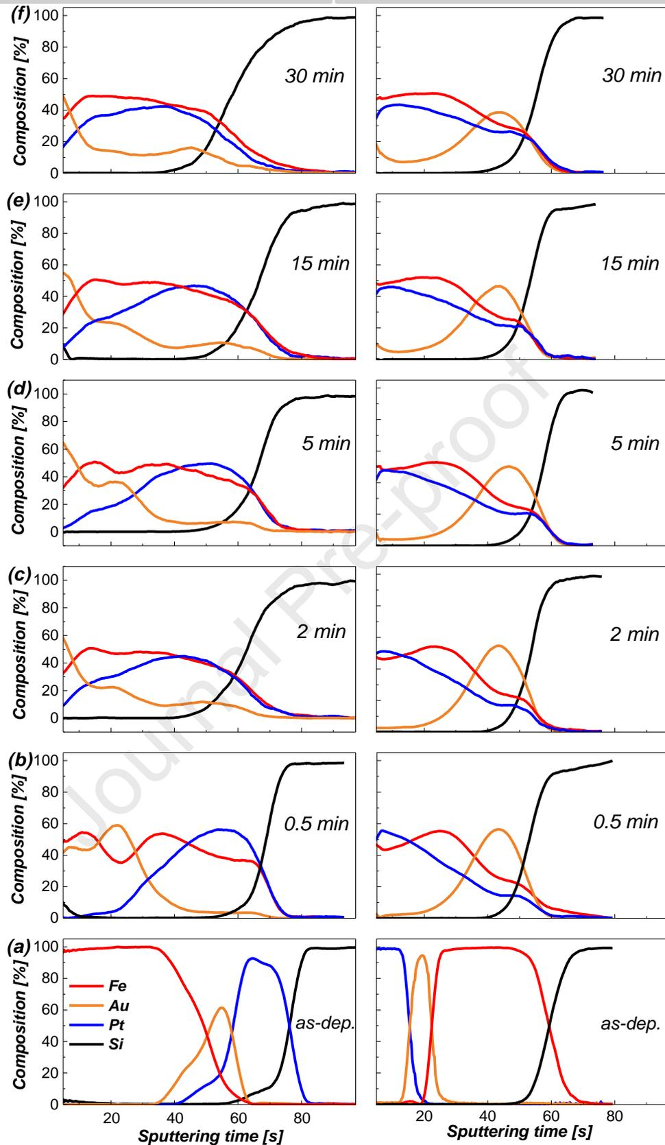
**Fig. 5.** Compositions versus sputtering time profiles of the (a) as-deposited Fe(15 nm)/Au(10 nm)/Pt(15 nm) and Pt(15 nm)/Au(10 nm)/Fe(15 nm) trilayers and (b-f) after annealing at 700 °C for different annealing times up to 30 min.
