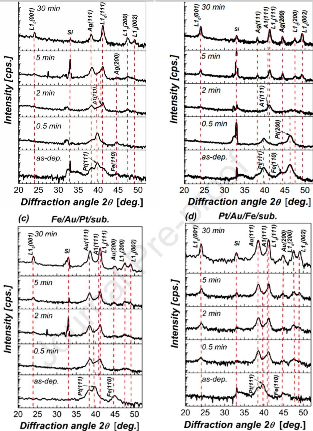
**Fig. 1.** X-ray diffraction patterns of as-deposited and post-annealed (700 °C for 0.5–30 min) trilayers: (a) Fe(15 nm)/Ag(10 nm)/Pt(15 nm), (b) Pt(15 nm)/Ag(10 nm)/Fe(15 nm), (c) Fe(15 nm)/Au(10 nm)/Pt(15 nm), and (d) Pt(15 nm)/Au(10 nm)/Fe(15 nm).
