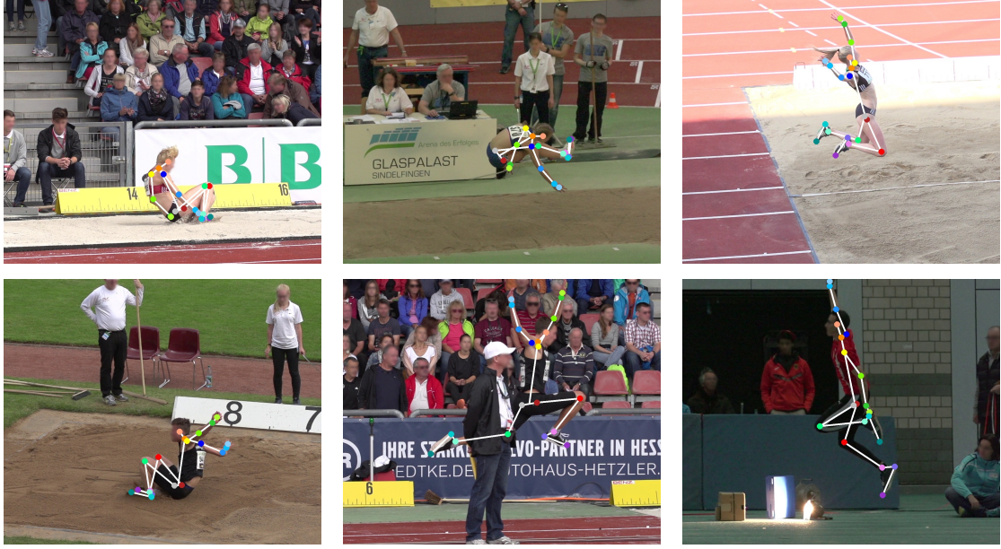
Figure 4.6: Example images with predictions from the model trained with pseudo-labels. It can deal with occlusions, extreme poses, and new keypoints like toe tip or heel, although such cases are not included in COCO.
