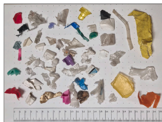
Fig. 1. Materials and Experimental set-up. (a) Chips: LDPE red/white (using VIS camera), (b) Flakes: PO/PET (using NIR camera), (c) Scheme of experimental set-up using a chute sorter with VIS and NIR camera and corresponding light sources.
