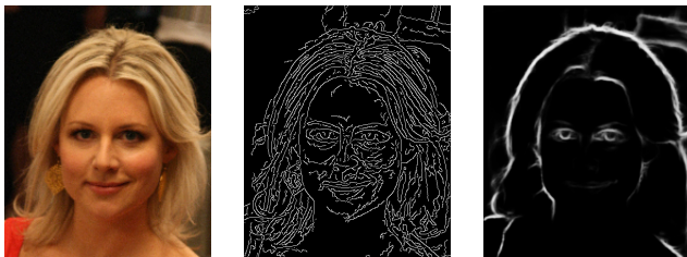
Figure 5. Edge transformations of the original image (left) using Canny edge detector [1] (middle) and HED [30] (right).
