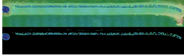
Figure 5. Segmentation of surface defects based on height profile
