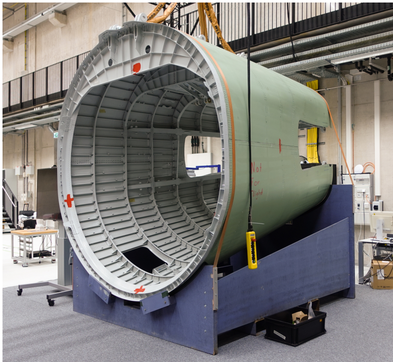
Figure 5.6. Partially assembled "Section 19" of an Airbus A320 Aircraft used for testing.
