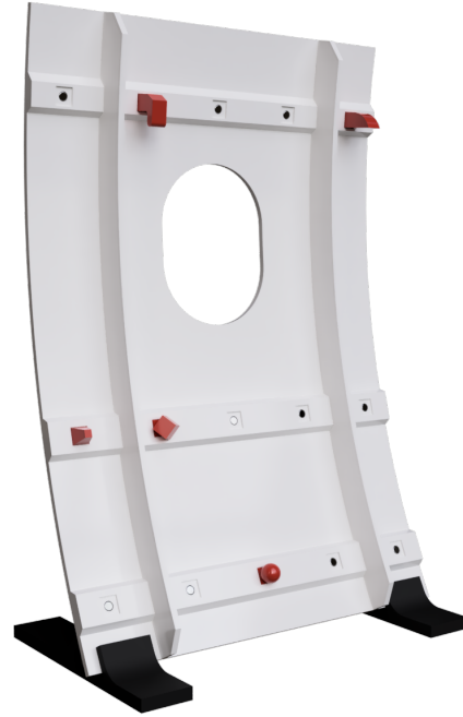
Figure 5.8. 3D-printed mockup of an aircraft fuselage part with reconfigurable mounting brackets.
