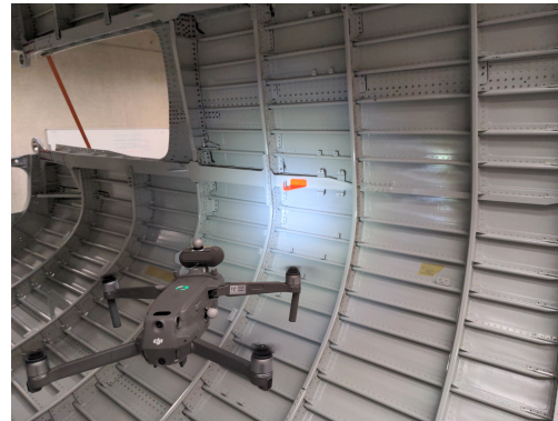
Figure 5.3. Headlight attachment illuminating inside of plane fuselage.
