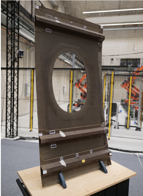
Figure 5.7. Cutout of center section of an Airbus A350 Aircraft.
