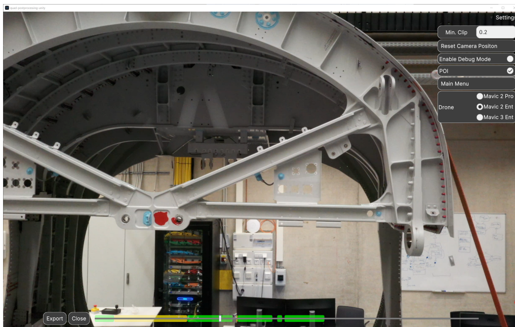
Figure 4.19. Custom Video Player for selective playback of an inspection flight.
