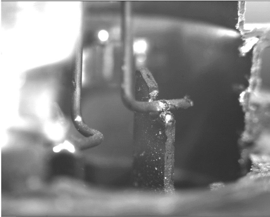
Figure 2.2: Electrode welded to the contact fin. The socket was sawed open for demonstration purposes.
